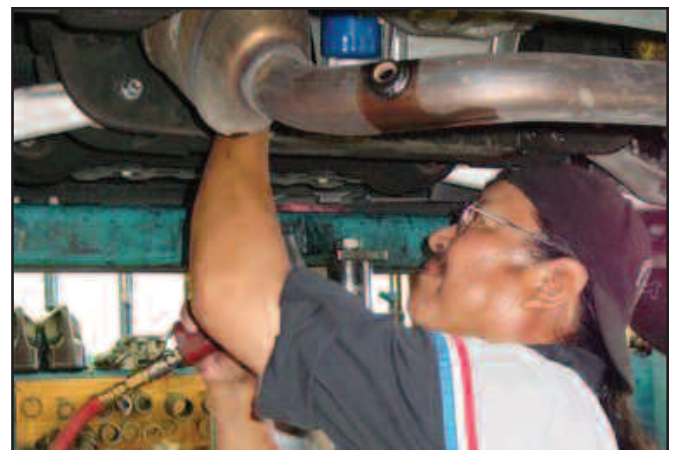
Harry Curley works on a GM transmission removal.
